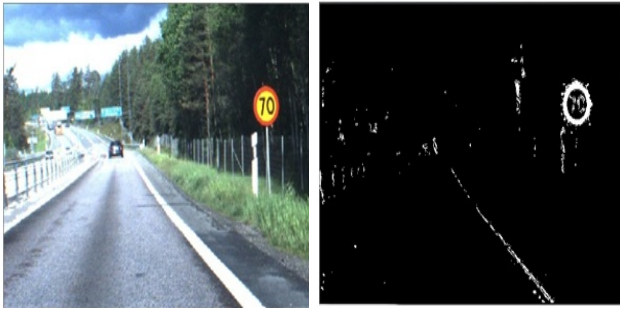
Fig. 3. Input image and image after thresholding
